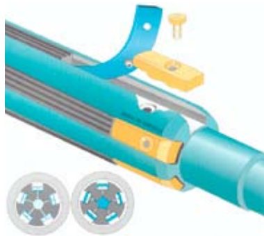
The picture shows how the air tubes are mounted in the air shaft.
